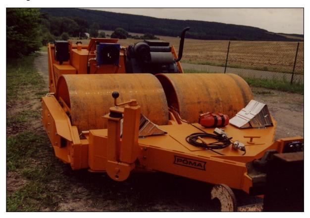
The PÖMA – ARW 200 is developed for compacting jobs in connection with road construction and maintenance work. The machine is working very economic on roads for forestry and agriculture.
